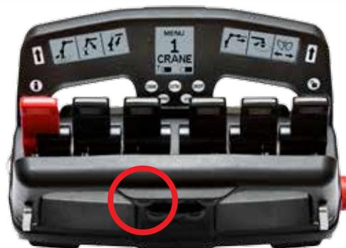
It is easy to switch between CTC and normal crane mode by pressing a button on HIAB's hand controller XSDrive (top) or CombiDrive (bottom).
